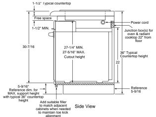
This installation is to achieve minimum gap between bottom of countertop and control panel.
